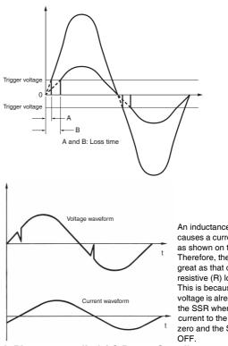
An inductance (L) load causes a current phase delay as shown on the left. Therefore, the loss is not as great as that caused by a resistive (R) load. This is because a high voltage is already imposed on the SSR when the input current to the SSR drops to zero and the SSR is turned OFF.
