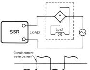
Accordingly, AC SSRs use a triac (which turns OFF the element only when the circuit current is 0 A) in the output element. If the load current waveform is rectangular, it will result in an SSR release error.
