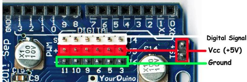
The **Black Sockets at the top** (Places you can connect wires and devices to) are numbered 0 to 13 from **right to left**. These are the **DIGITAL INPUT/OUTPUT** connections. You can push wires or the pins on the end of wires into those "Black Holes" and connect them to many different devices. That's the traditional Arduino way. But it's easier to use the Robo1 connector pins.
