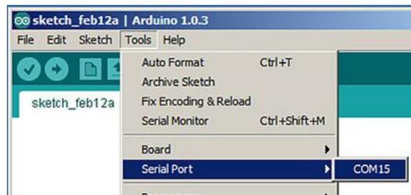
On the MAC, see the example on the right. Pick the entry that has both "tty" and "usbserial" in it.
