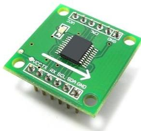
This is a digital compass module with UART and IIC interface, 3-5V voltage supply , it's very easy to work with may controller.
